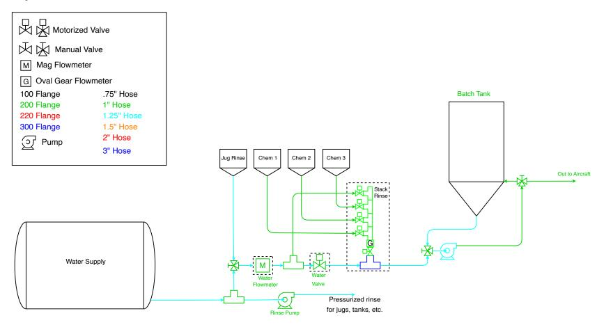
Mixmate components are marked with the dashed box.
